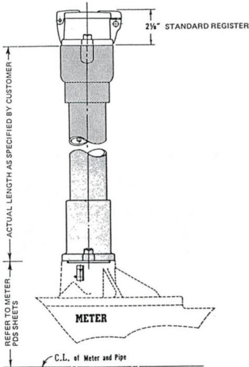
This rigid extension is suggested for pit or other installations to raise the register clock to a more convenient level for reading and servicing. The extension is coupled directly to the meterhead, replacing the original register clock. Installation can normally be completed in the field without removing the meter from the line. The original register clock is relocated on top of the extension.
