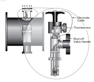
The second is the "hot-tap" electrode which allows electrode replacement while the system is still under pressure without disturbing the process flow. Removal can be easily performed with a phillips screwdriver and a crescent wrench. Special locking catches were designed to prevent high pressure accidents during electrode removal. The shut-off valve must be closed before the electrode may be removed.
